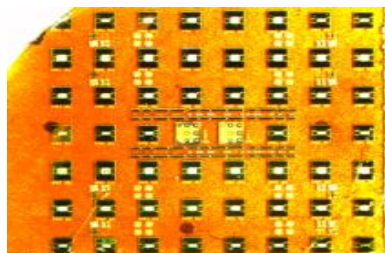
GaN HEMT structures on GaN wafer
